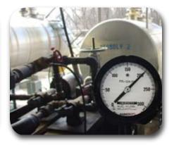
The LVP series develops up to 14 Bar (200 PSI) on thin, corrosive liquids, where gear pumps and other manufacturer's vane pumps are limited to 8.5 Bar (125 PSI) or less. The reduced slip characteristics of Viking's LVP pumps provide enhanced self-priming and suction lift capabilities.
